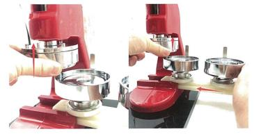
Step 4: hold up the upper mold, make sure there is no gap in the upper mold. Then sliding mold slide to the body groove.
