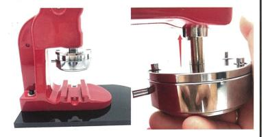
Step 3: set into upper mold. Align the bump with the groove.
