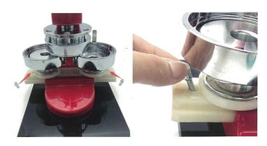
Step 5: put two nails in holes to secure the mold.
