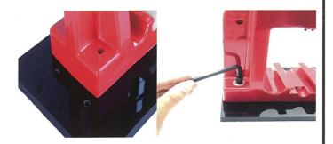
Step 1: use  $\Phi 6$  Allen key to screw body and base plate with a bolt and a washer.
