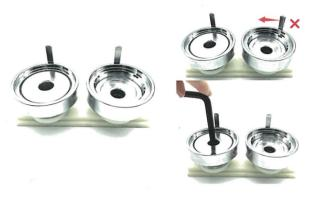
Step 2: check the mold, make sure two baffles on the middle position. If the baffles is shifting, rotating the mold to the middle position and use  $\Phi$  8 Allen key to fasten it.
