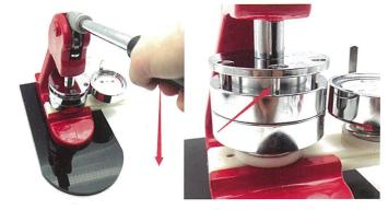
Step 3: press down the handle. Make sure there will be some gap in the upper mold when you press the left mold.
