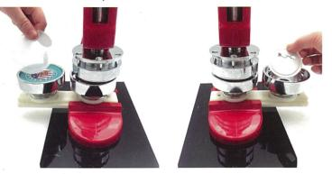
Step 2: place plastic film on circular printing paper. Then sliding mold slide, place plastic pin badge on right mold.
