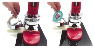
Step 1: place metal tin shell in left mold. Then place circular printing paper on metal  $_{\rm t}$ in shell. The paper size should be the same size to the plastic film.
