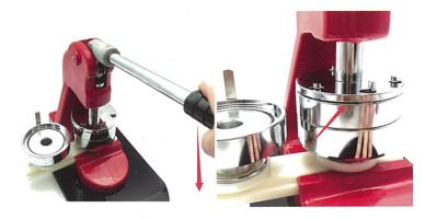
Step 4: sliding mold slide, press down the handle. There must be no gap in the upper mold when press the right mold.
